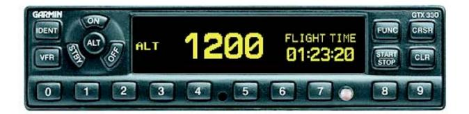
It operates on radar frequencies, receiving ground radar interrogations at 1030 MHz and transmitting a coded response of pulses to ground-based radar on a frequency of 1090 MHz. The GTX 330 is equipped with IDENT capability that activates the Special Position Identification (SPI) pulse for 18 seconds. Mode S transmit/receive capability also requires 1090 MHz transmitting and 1030 MHz receiving for Mode S functions.
